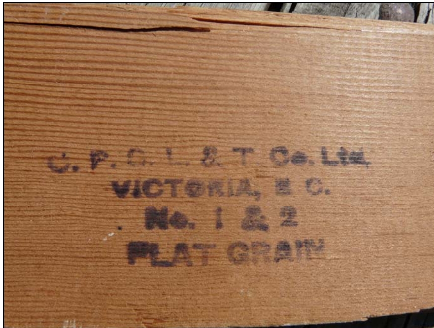
Stamp on fir lumber found during renovation material salvage. (Andy Blicq)
