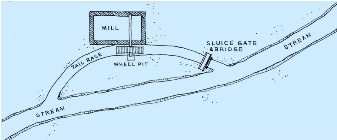
This sketch plan shows an imaginary mill situated on generally flat ground, and thus with a trench that is used to divert water from the main stream course. A sluice gate and bridge shown at the right-hand side were used to control water volumes that entered into the trench.
