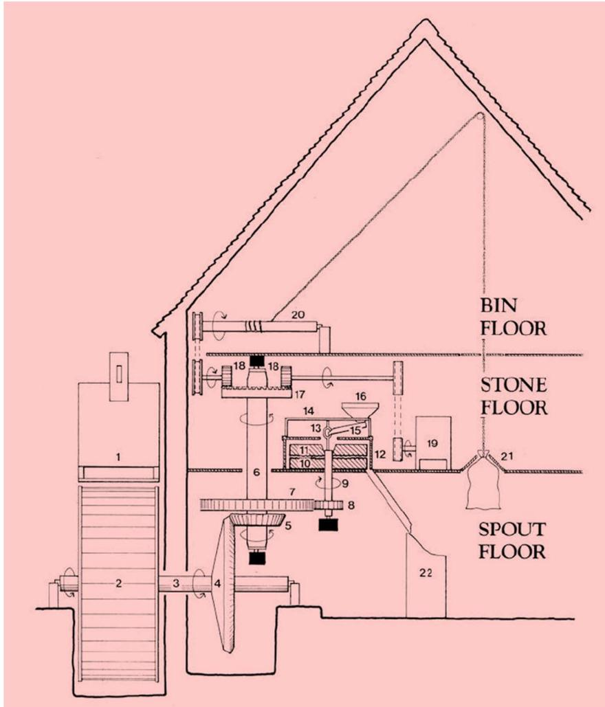
This image describes a more complex operation than obtained at John Gunn's mill, but it does provide a clear graphic sense of some key parts of mechanisms and of likely operations: the water wheel (2) on the large axle (3) turning the large gear (4) which engages other gears (5, 7 and 8) and finally the smaller axle (9) that turns the millstones (10 and 11). Different sizes of gears were used to gradually reduce and refine power levels to the grinding stones.
