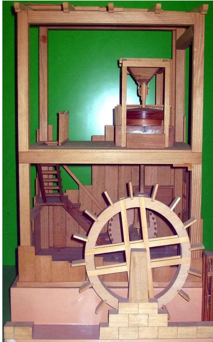
Model of a Roman type water-powered grain-mill described by Vitruvius. The millstone (upper floor) is powered by an undershot waterwheel by the way of a gear mechanism (lower floor). This essential mechanical organization will be seen later in Mr. Gunn's mill.
