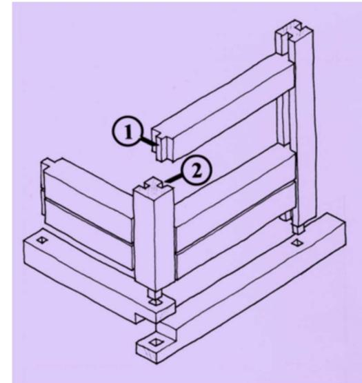
The distinctive quality of Red River frame is presented in this detailed cutaway view of a typical corner connection. The tongue (1) on the horizontal log is slipped into the groove (2) chiselled into the vertical log.
