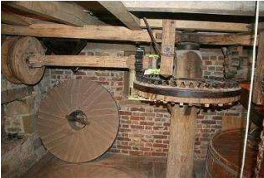
The interior of a functional watermill at Weald and Downland Open Air Museum in England. This image shows the various wooden axles, wheels and gears required in a grist mill operation. The large circular stone leaning against the brick wall is one of the grind stones required in a flour milling operation.
