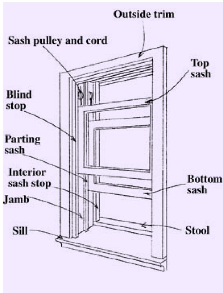
This rendering suggests the complexity of window construction and operating technologies. It is presumed that the production of the James White factory would only have provided the simplest of sash windows – mostly without pulleys and weights.
