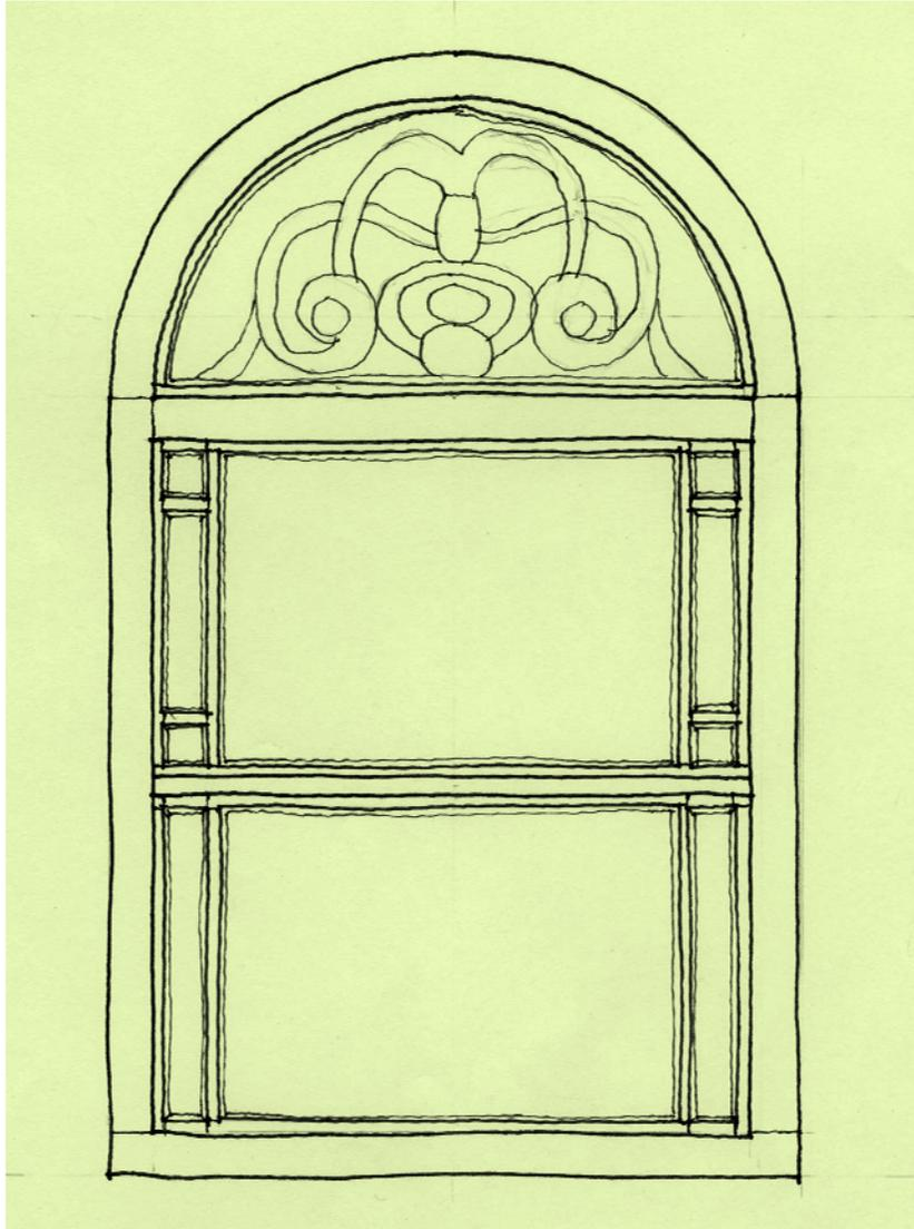
A sketch of one of the windows still present in the White Sash and Door Factory. Some of James White's windows can be identified by the common use of side glazed panels that created a frame around the sash,
