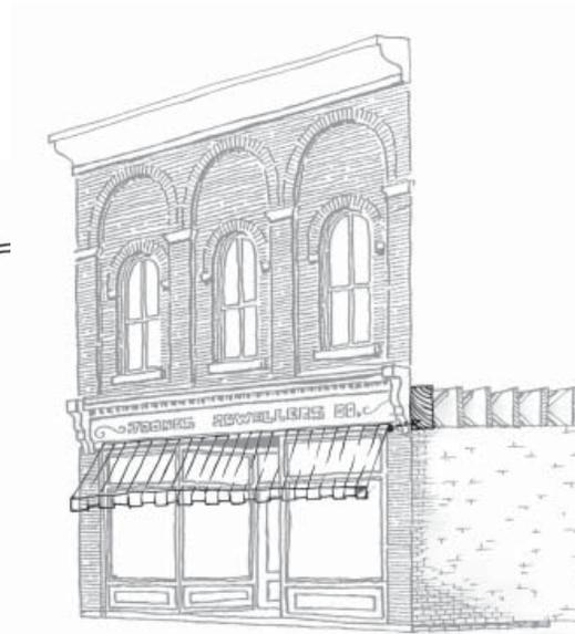
The awning is anchored to the structural beam behind. The beam is transferring the load of the second floor facade to masonry piers on either side of the glass storefront. A store front fascia sign rests above.
